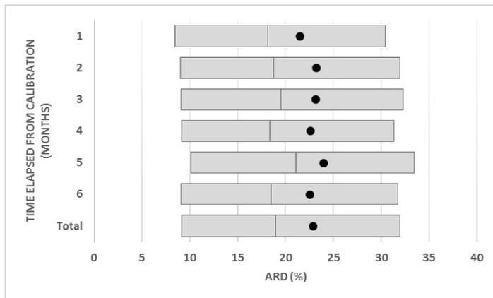
**Figure 3:** Device performance expressed as ARD (%) as a function of time elapsed from calibration. The left side of the boxplot represents quartile 25%, the middle line represents the median, and the right side quartile 75%. Black dots represent mean ARD.
